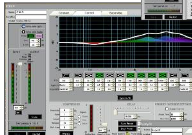
Individual Control windows for each Iconyx-R array allow easy adjustment of EQ, Shelving, Delay, Etc.
