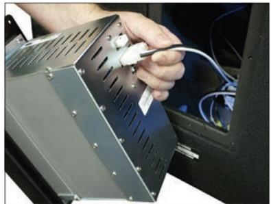
Note that this bypasses the Crossover Network and it no longer will have any effect on the subwoofer's performance. The output of the amplifier is now connected directly to the woofer and RHAON is now in control of the subwoofer's performance.
